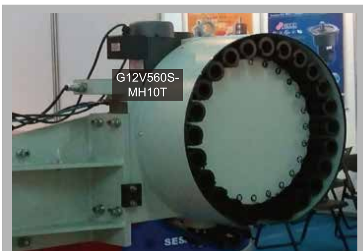
G12V560S-MH10T用於刀庫圖示 G12V560S-MH10T on ATC.
